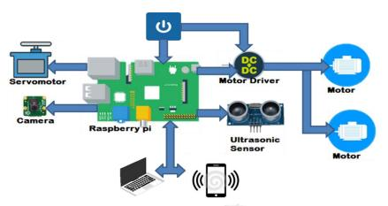
FIGURE 1: System schematic layout.
