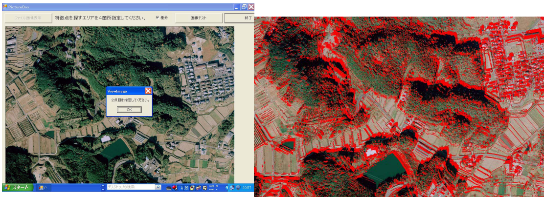
(a) Screen shot image for manual extraction (b) Difference between two satellite images of tie points which are acquired on before and after
