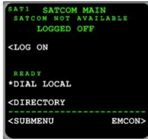
FIGURE 21: The SDU (Level D) Interacts with the MCDU ( Level A Component Present in the Cockpit).
