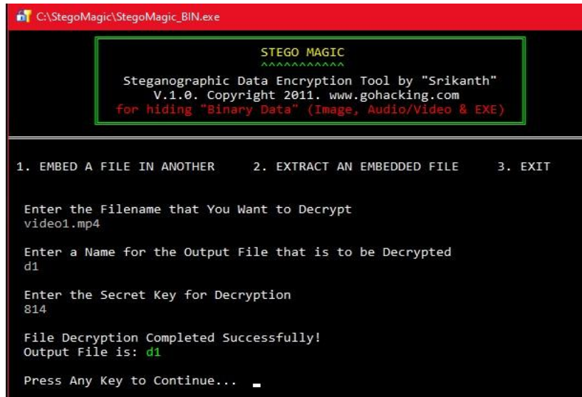
FIGURE 19: The Extraction Process in StegoMagic.
