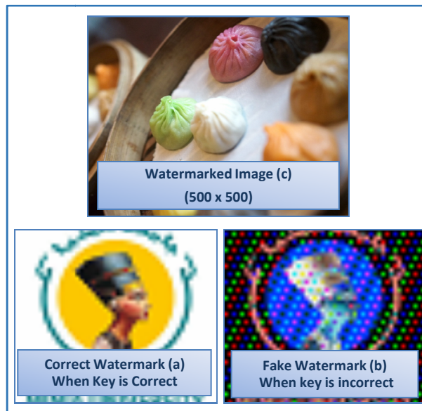
FIGURE 4.2: Watermark Extraction using Modified MSLDIP when input can be correct key and incorrect key.
