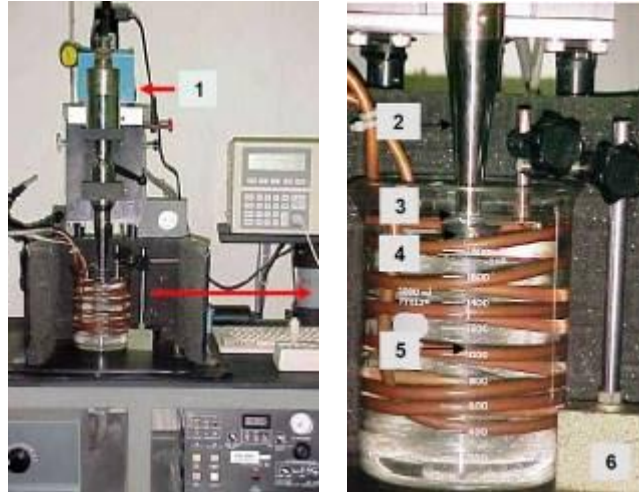
FIGURE 5: Experimental bench and assembly detail, 1 - system for adjusting the sample height by means of micrometer, 2 - sonotrode, 3 - stainless steel counter body (AISI 304), 4 - sample, 5 - cooling system, 6 - sample holder.
