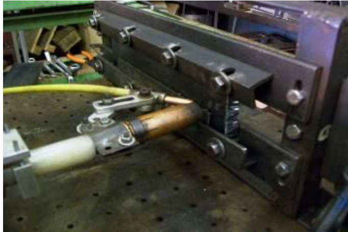
FIGURE 3: Experimental assembly for the GMAW process cold wire, with horizontal torch in the neutral position.
