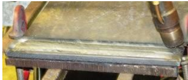
FIGURE 2: Welded coating in the flat position by the MIG / MAG double wire process.
