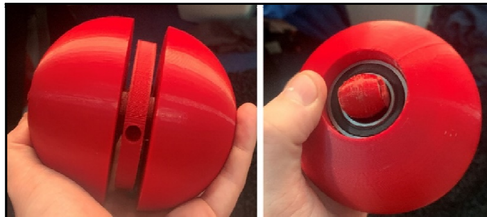
FIGURE 5: The integrated omni ball (left panel) combined with the small wheel (right panel).
