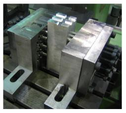
**FIGURE 1**: Prototype of Pin Type fixture
