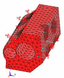
FIGURE 5: Sample workpiece evaluated using FEA for final clamp configuration
