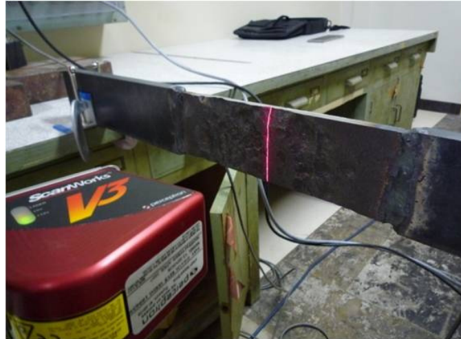
FIGURE 2: Condition of thickness measurement.
