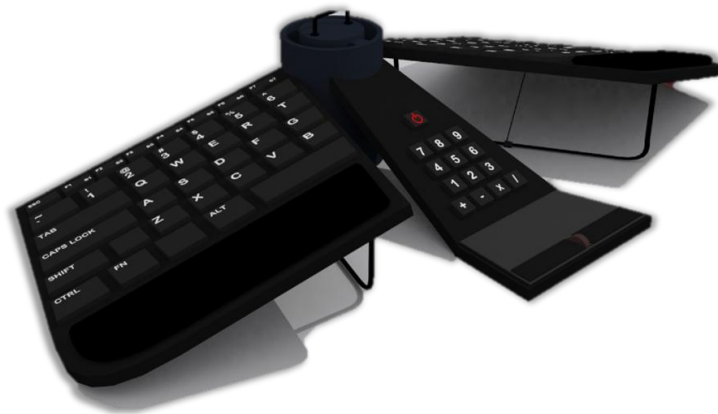
FIGURE 10: Trinity keyboard design in the tented position displaying its tilting feature
