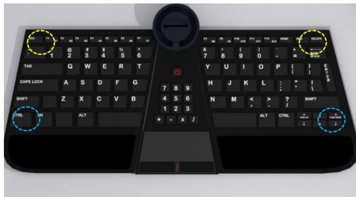
FIGURE 9: Trinity keyboard design in standard position. Dashed circles indicate the kickstand placement that is behind the base. The yellow circles represent rear stand set. The blue circles represent the front stand set closest to the user.
