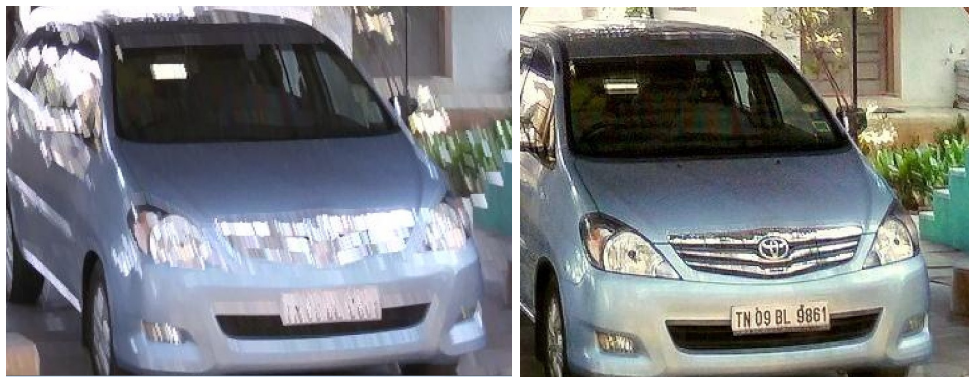
FIGURE 9: Close up of the car. In the original image the registration number is not clear (left) whereas in the fused output (right) it is clearly visible.
