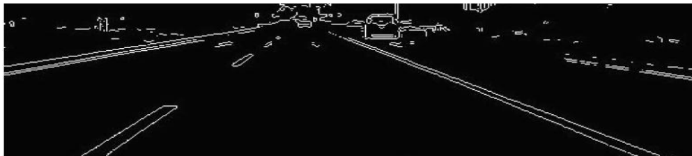
FIGURE 6: Canny Edge Detection Output image [1].
