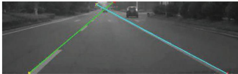
FIGURE 8: Lane detection output after Hough transform [1].
