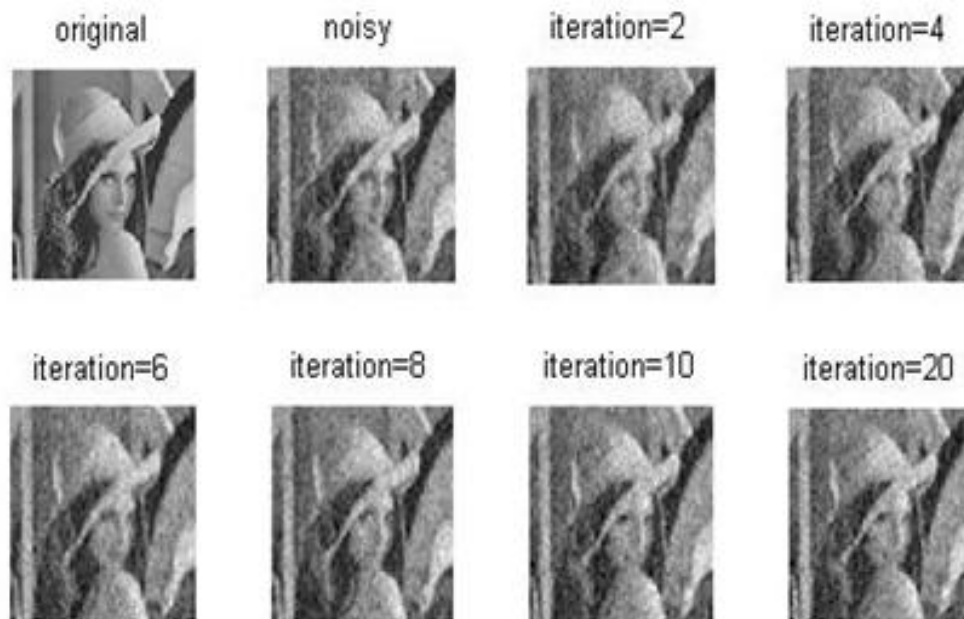
FIGURE 2: The results of de-noising “Lena” by the CoSaMP algorithm using different iterations and CR = 0.5 .
