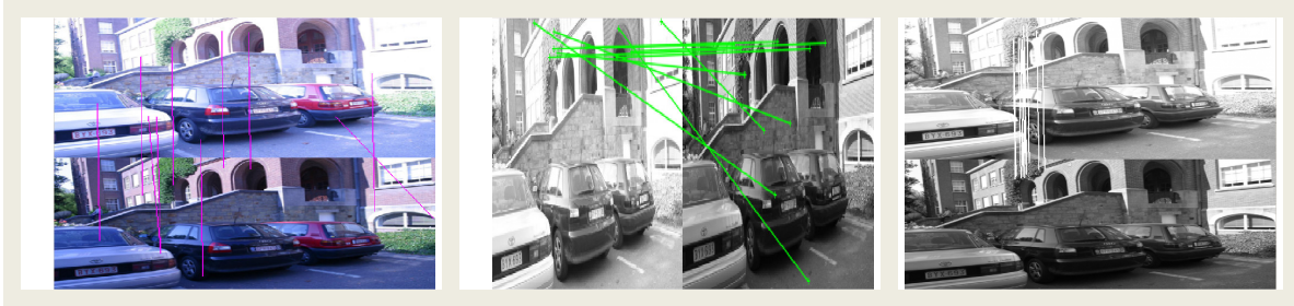
FIGURE 7: Illumination changes comparison. Using group G of figure 1, from left to right, SIFT (9 correct / 10), PCA-SIFT (6 correct / 10), SURF (10correct/10).
