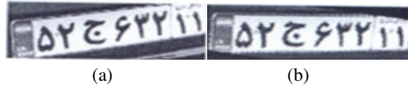
FIGURE 9: (a) the image before rotation and (b) rotated image after rotation adjustment.
