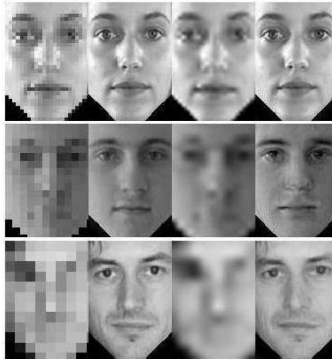
FIGURE 8: Hallucinated faces with the Eigen transformation in wavelet domain. Input, original, Bicubic interpolated and hallucinated images. For magnification factors of four (top), eight (middle) and eleven (bottom).
