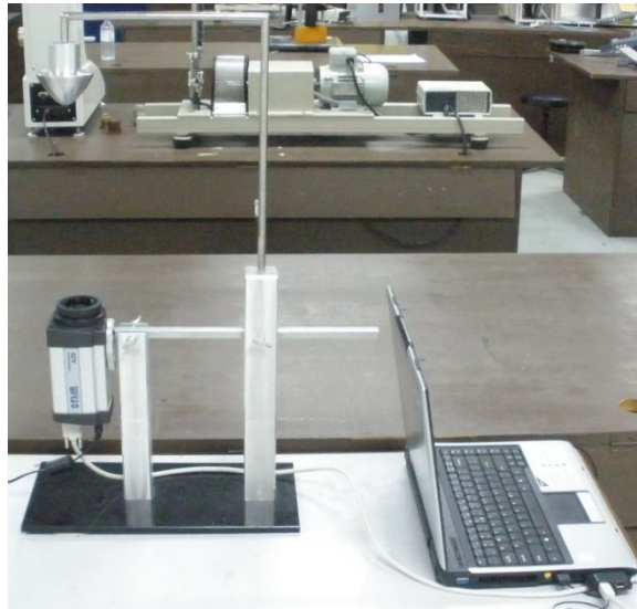
Fig. 2: Overall Fabricated Omnidirectional Thermal Visualization System Model
