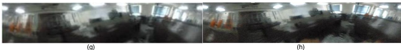
Fig. 20: Output of digital image using different mapping technique (a) point sample (b) mean (c) nearest neighbor interpolation of point sample (d) nearest neighbor interpolation of mean (e) bi-linear interpolation of point sample (f) bi-linear interpolation of mean (g) bi-cubic interpolation of point sample (h) bi-cubic interpolation of mean
