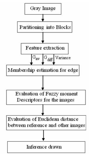
Figure 1: Basic steps involved in the recognition process
