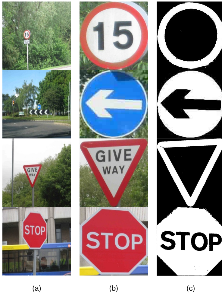
FIGURE 10: Colour Segmentation using HSV colour space (a) Road Signs in the natural environment (b) Cropped Road Signs from the original Image (c) Cropped Road Signs from the Binary Image
