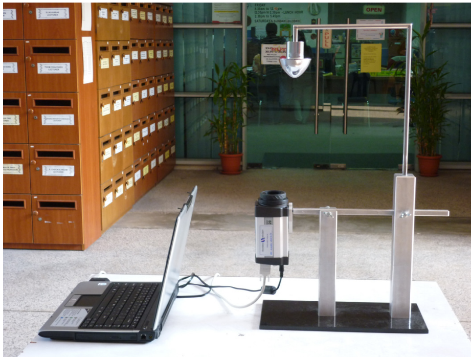
FIGURE 4: Overall fabricated omnidirectional thermal imaging surveillance system model
