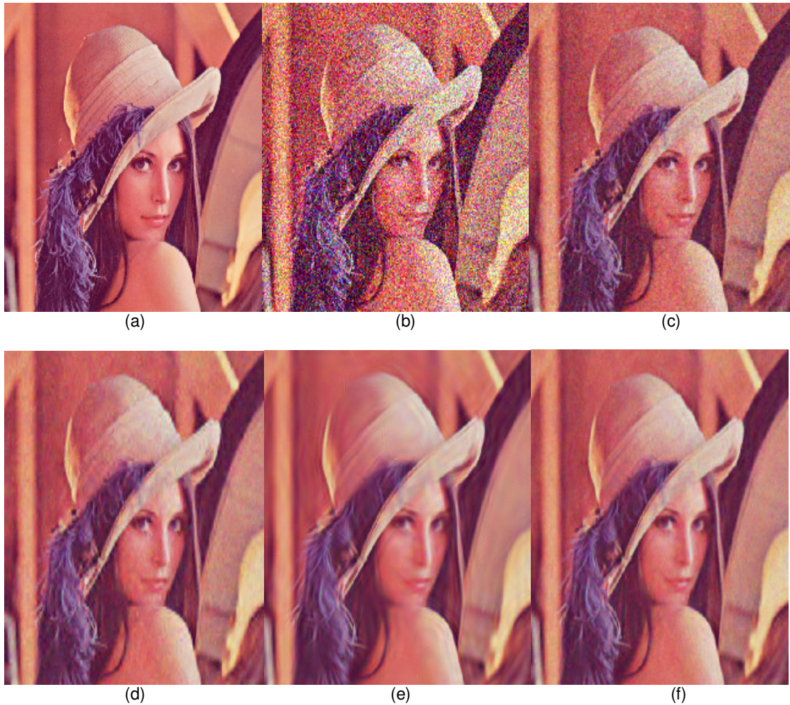
FIGURE 4: Lena colour test image: (a) Original image, (b) Noisy image with \sigma = 50 dB, (c) Image after denoising with Gaussian filter , (d) Denoised image from BayesShrink Wavelet Thresholding, (e)Denoised image from Curvelet transform, (f)Denoised image from Proposed method.
