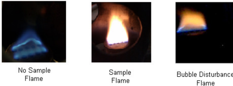
Figure4: Captured Flame Details
