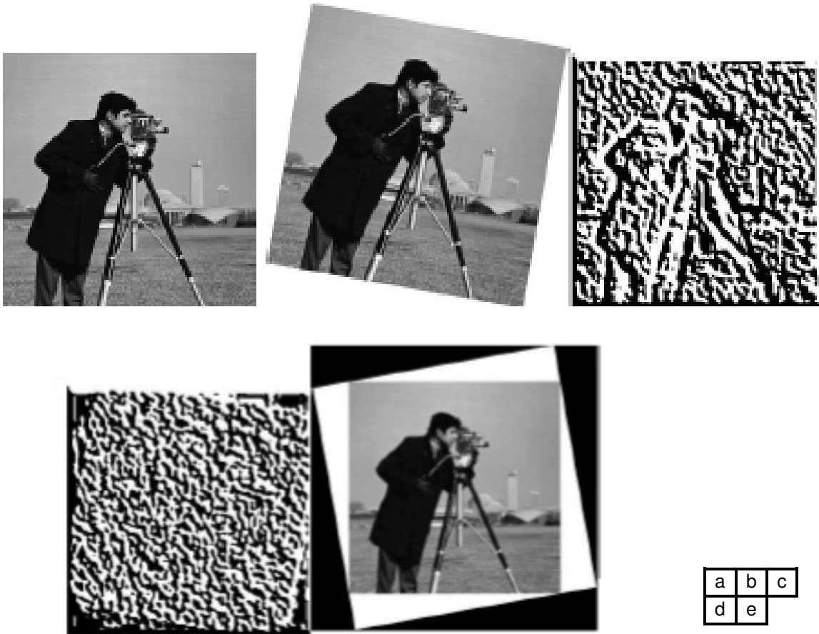
FIGURE 4.9: (a) Reference Input Image (256X256 ) (b) Image 2: Rotated Image ( 296X296) (c) Transformed Reference Input Image (256X256) (d) Transformed Image 2: Rotated Image ( 296X296 ) (e) Registered image ( 256X256 ).
