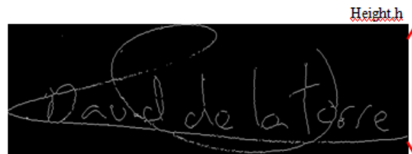
FIGURE 7: The value of height can be obtained by scanning from top to bottom of the image.
