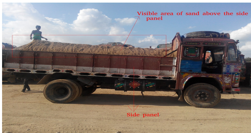
FIGURE 1: Explains the positioning of side panels and the visible area of sand concept.
