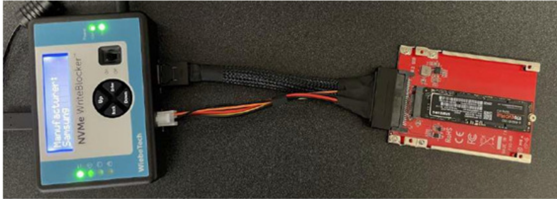
FIGURE 4: Silicon Power NVMe SSD attached with NVMe WriteBlocker.
