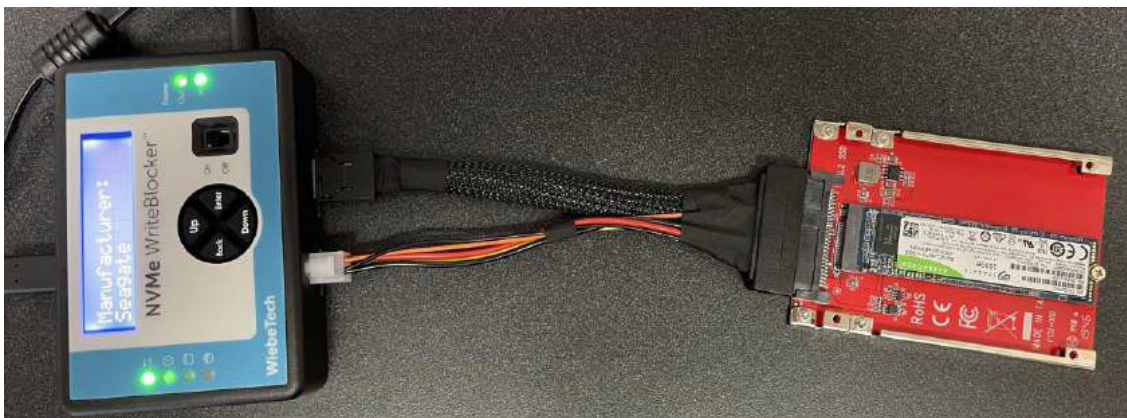
FIGURE 2: Seagate NVMe SSD attached with NVMe WriteBlocker.
