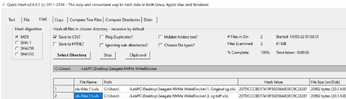
FIGURE 12: Hash values of xls-files(1).xls in Seagate NVMe SSD when using NVMe WriteBlocker.
