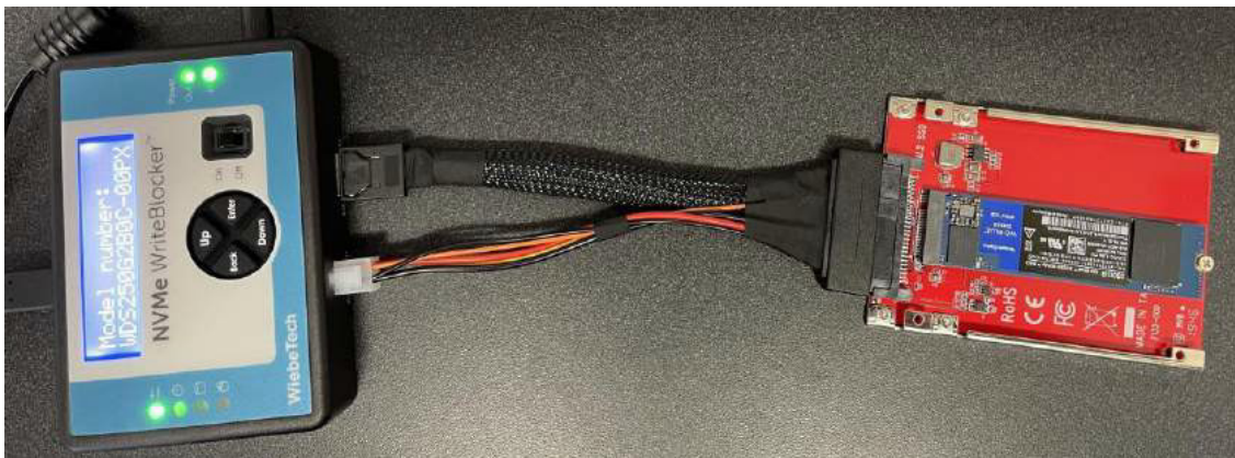
FIGURE 3: Western Digital NVMe SSD attached with NVMe WriteBlocker.
