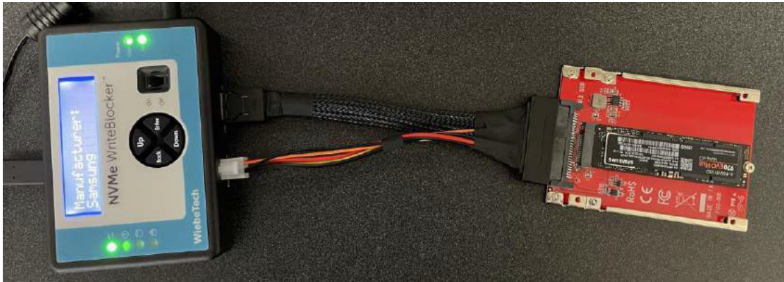
FIGURE 1: Samsung NVMe SSD attached with NVMe WriteBlocker.
