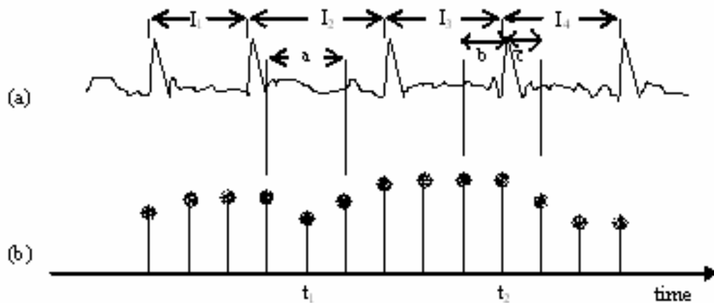
FIGURE 1: Berger's method of interpolation. Where a, b, and c are the local windows; I_1, I_2, I_3, I_4 are the distance between RR-peaks; t_1, t_2 are the time points.
