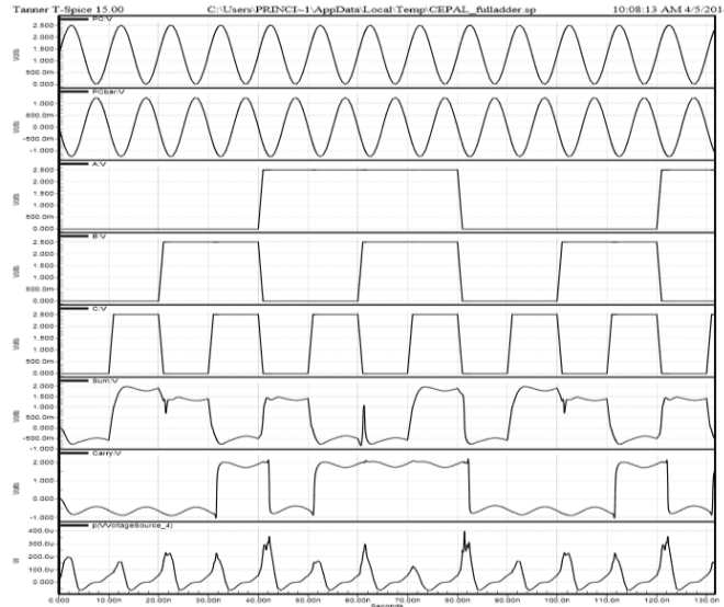
FIGURE 5: Output waveforms of Full Adder.
