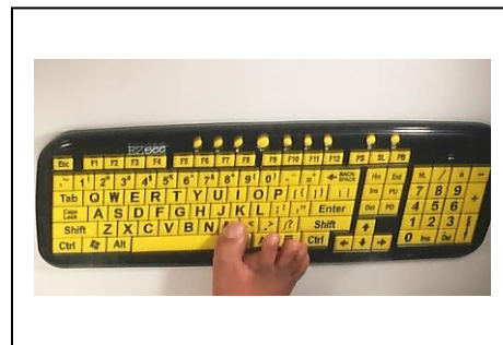
FIGURE 9: Toe is pressing the letter 'M'. The image is a reflected image that appears in front of the user. The keyboard was lit by the LED light sources(Khan, et al., 2019).
