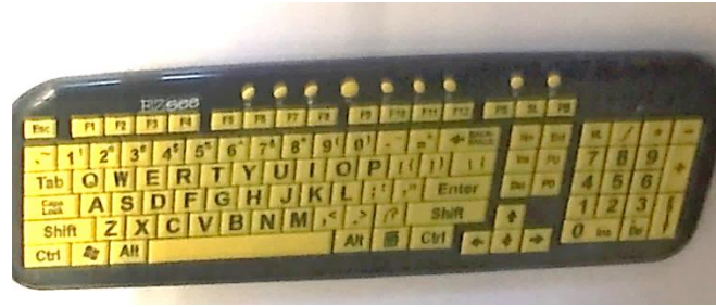
FIGURE 10: The reflected image of a high contrast keyboard with large letters. All the letters are visible and easily recognizable in the reflected image. The room light source is located on the left side of the keyboard; this is why, the left side of keyboard looks brighter than the right.
